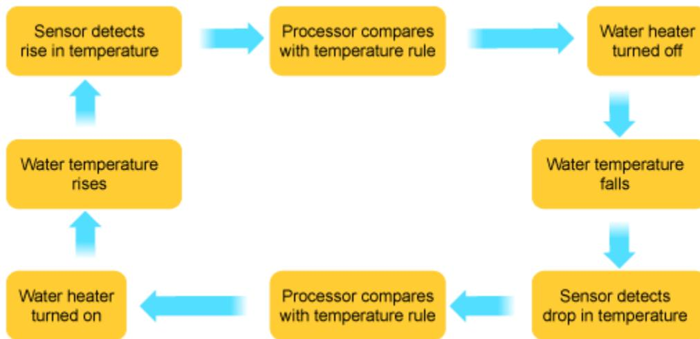
A system that monitors the water temperature of a fishtank and reacts accordingly.
